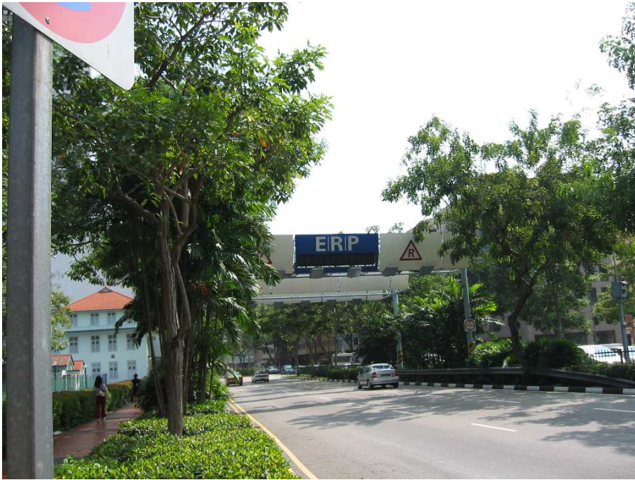
Figure 2.9: Picture of a gantry of the electronic road pricing (ERP) system in Singapore. Vehicles are detected and tolled according to the time of day and the chosen route.
