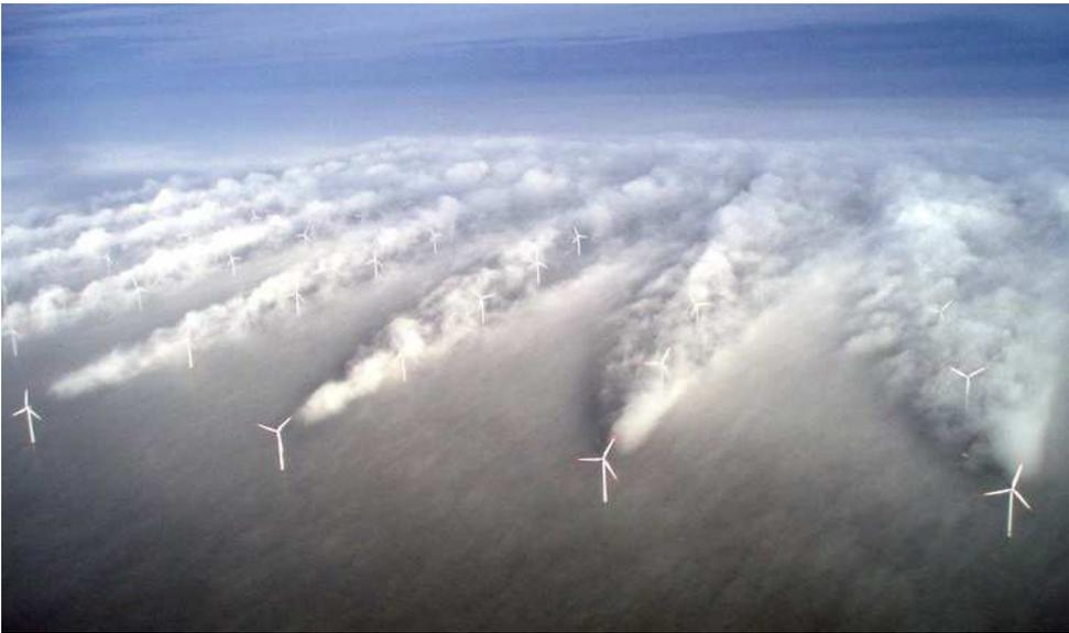
Figure 1.1: Clouds forming in the Horns Rev offshore wind plant in Denmark, showing the flow structures behind each turbine (the wind turbine wakes), that cause interaction with the turbines downstream. Source: Christian Steiness. See also Hasager et al. (2013) for more information on the picture.
