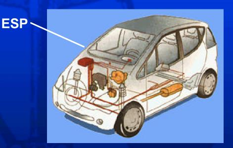
Unstable behavior improved by Electronic Stabilization Program (ESP)
