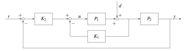
The signal *r* is the reference signal, *d* is a noise signal, *y* is the output of the system, and *u* is the input signal for system  $P_1$ .
