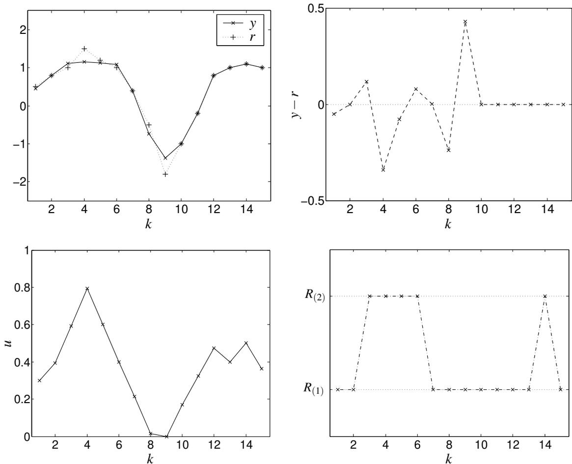
Figure 1: The closed-loop MPC output signal  $y$ , the reference signal  $r$ , the difference signal  $y - r$ , the input signal  $u$ , and the region  $R_{(i)}$  (cf. Footnote 10) in which the system is at sample step  $k$  for Example 6.1.
