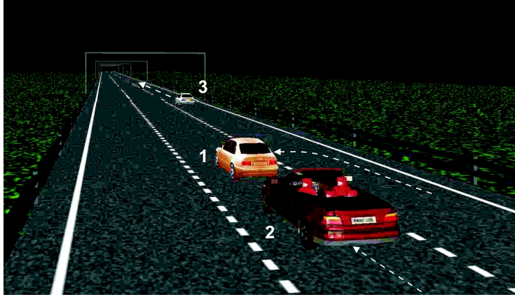
Figure 7. Visual representation of a cut-in scenario in the virtual world: the ACC-equipped vehicle (2) drives on the middle lane when suddenly a vehicle (1) cuts in from the right lane at a lower speed.
