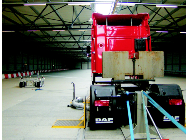
Figure 13. Experimental setup of a VEHIL test with a truck, equipped with an FCW system.
