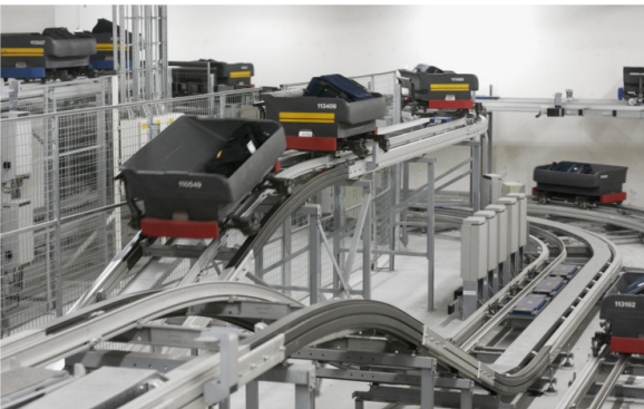
Figure 1 DCVs running on a network of tracks. Photo courtesy of Vanderlande Industries.
