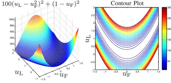
Fig. 3. The Rosenbrock function and several level curves.
