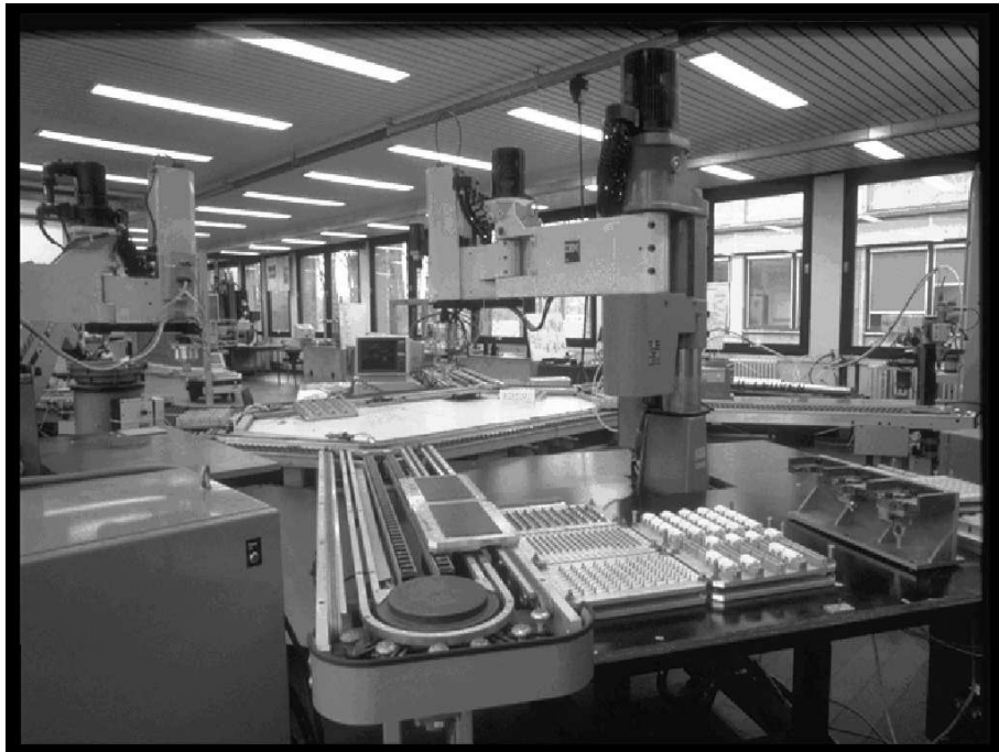
Figure 2: The PMA flexible assembly system testbed.
