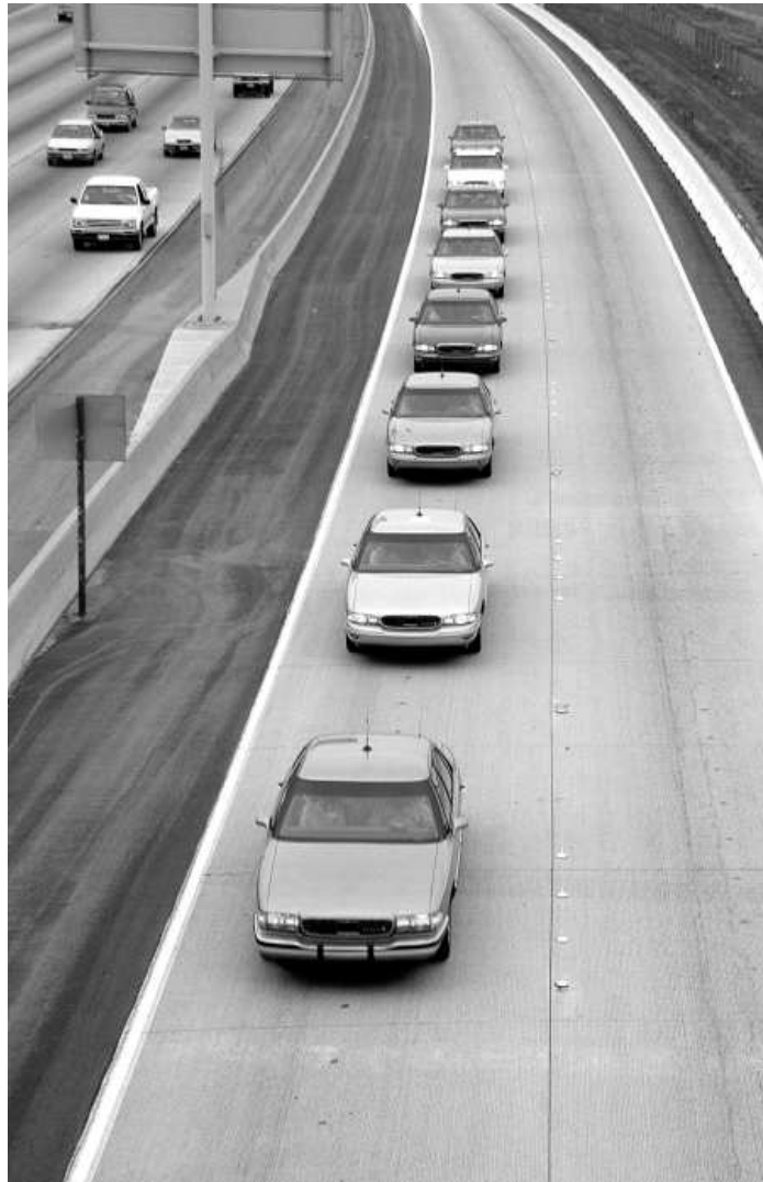
Figure 1: Snapshot of the demonstration of automated highway system technologies by the National Automated Highway System Consortium held in San Diego, California from August 7–10, 1997 [5]. In this demonstration eight vehicles travelled in close coordination under fully automated longitudinal and lateral control. The cars maintained a fixed spacing of 6.5 m between themselves at all speeds up to full highway speed. (Photo courtesy of California PATH)
