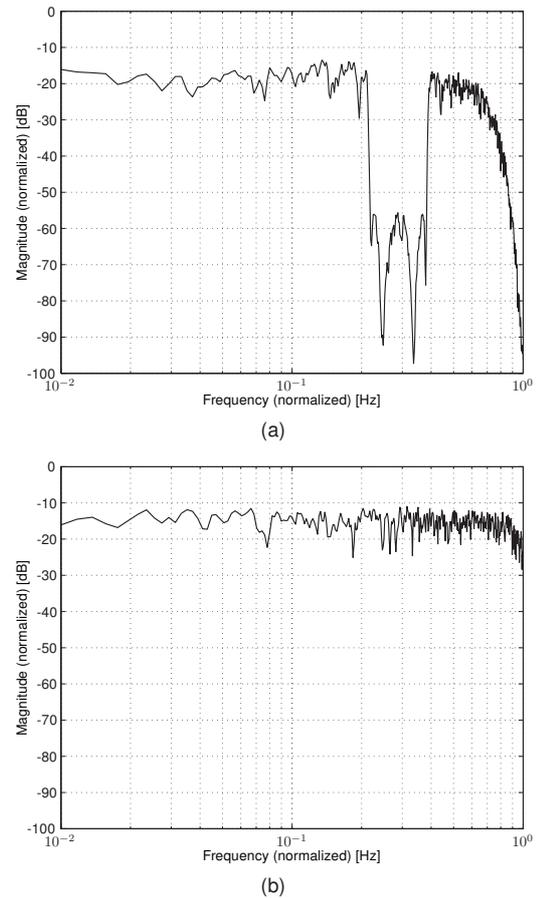
Figure 2: Spectral density diagrams of the additional excitation signals on the pitch (a) and the generator torque (b) inputs.
