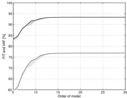
Figure 4: The mean FIT (grey) and VAF (black) against the order of the model identified with VARX-based PBSID. The grey region shows the errorbounds for the models of 100 Monte Carlo simulations. ( $p = 50, f = 15$ )
