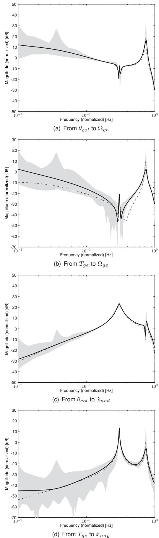
Figure 6: Bode diagrams of the TURBU model (dashed) and the identified model with the highest VAF value (bold). The other 99 models are within the grey region. ( $n = 16$ ,  $p = 50$ ,  $f = 15$ )
