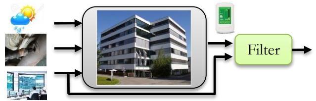
Fig 2: Fault detection filter fed by available measurements in an online operational mode
