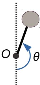
The angle  $\theta$  is equal to 0 when arm is in the bottom position and is equal to  $\pi$  in the upright position.
