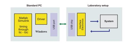
Possibly more sampling period jitter in the beginning of experiment – in case of suspicion, discard a few initial samples.
