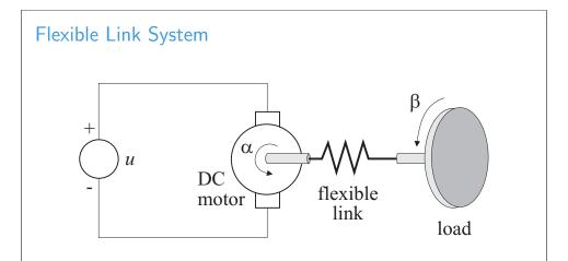
Abstraction of many real-world systems, such as robot arms, motors with gears, etc.
