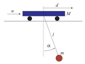
Figure 1: A schematic diagram of the container crane.
