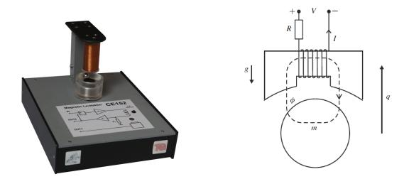
Figure 1: Left: a photograph of the magnetic levitation setup. Right: a schematic drawing.
