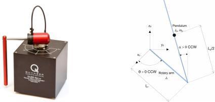
Figure 1: Qube-Servo setup and its schematic representation.
