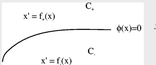
$$\phi(x)=0 \qquad \dot{x} = \begin{cases} f_{+}(x) & \text{if } x \in C_{+} := \{x \mid \phi(x) > 0\} \\ f_{-}(x) & \text{if } x \in C_{-} := \{x \mid \phi(x) < 0\} \end{cases}$$
