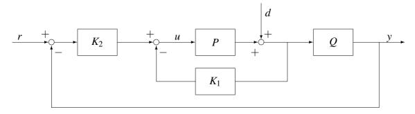
The signal r is the reference signal, d is a noise signal, y is the output of the system, and u is the input signal for system P.
