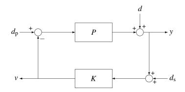
There are two output signals (y(k) and v(k)) and three disturbance signals  $(d(k), d_p(k), and d_s(k))$ .
