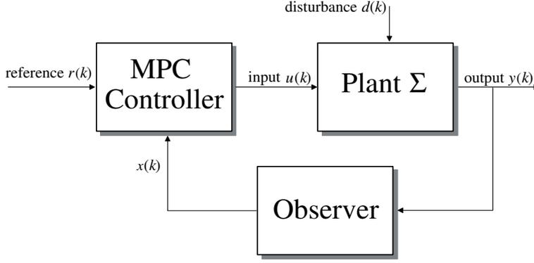
Figure 1: Closed-loop model predictive control system
