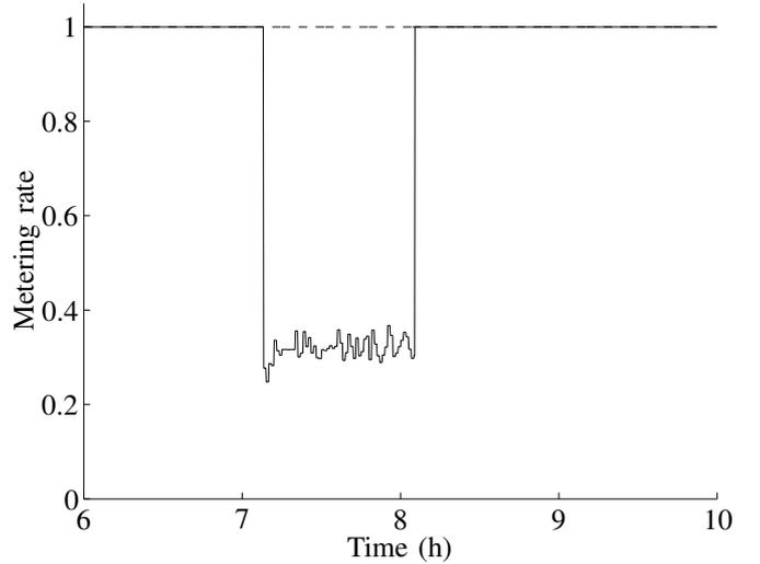
Fig. 6. Plot of the evolution of the metering rate as presented by both controllers. The solid line represents the controller using the correct model parameters ( $\beta_{\text{ref}}$ ). The dashed line represents the controller using the perturbed parameter set ( $\beta_{\text{pert}}$ ). Note that the controller with the perturbed parameter set never becomes active.
