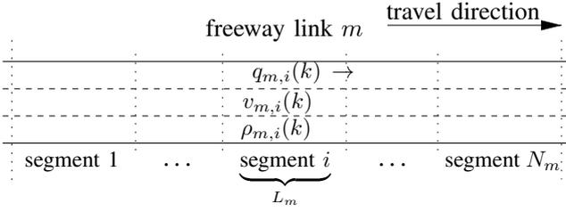
Figure 3. In the METANET model, a freeway link is divided into segments. The main variables in the model are the average outflow of a segment  $q_{m,i}(k)$ , the average speed  $v_{m,i}(k)$ , the average density  $\rho_{m,i}(k)$ , and the segment length  $L_m$ .
