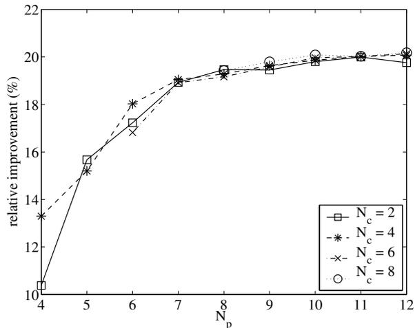
Figure 7. The relative improvement of the performance (Total Time Spent) in the continuous, unconstrained case compared to the no-control case as a function of  $N_p$  for several values of  $N_c$ . The sensitivity to  $N_p$  is much higher than that to  $N_c$ .
