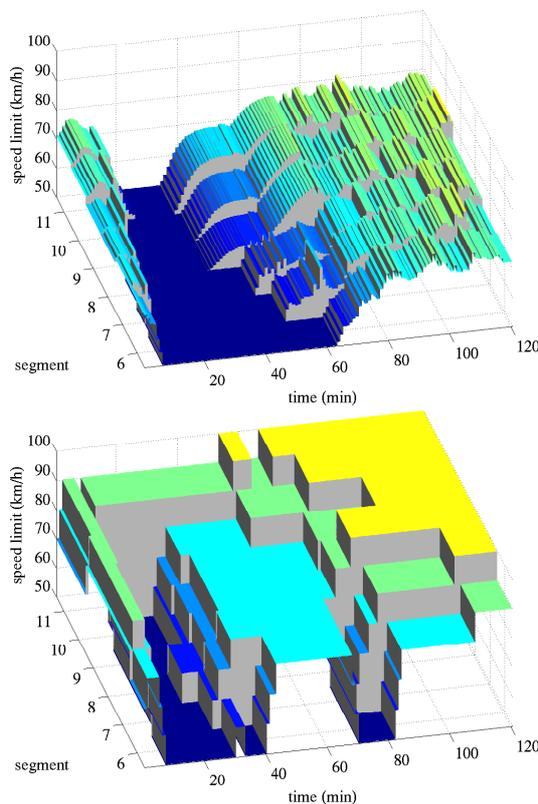
Figure 8. The speed limits for the continuous case without safety constraints and  $N_p = 10$ ,  $N_c = 8$  (top). The speed limits for the discrete (“ceil”) case with safety constraints and  $N_p = 10$ ,  $N_c = 8$  (bottom).
