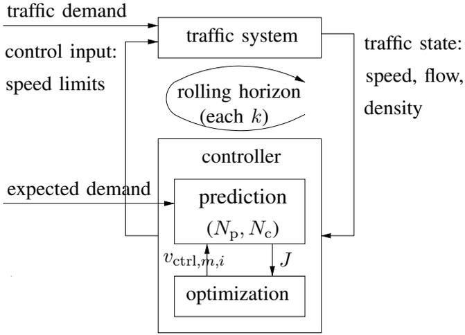
Figure 2. Schematic view of the model predictive control (MPC) structure.
