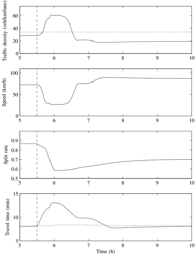
Fig. 8. Simulation results for anticipative MPC-based ramp metering. The plots at the top give the density and average speed in the first segment downstream of the on-ramp. The dotted line in the upper plot represents the critical traffic density  $\rho_{\text{crit}}$ . In the lower plot the instantaneous travel time is shown for the primary (solid line) and the secondary (dotted line) route from the mainstream origin to the destination.
