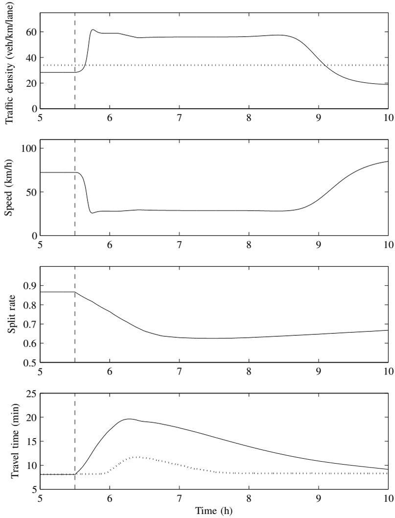
Fig. 6. Simulation results of anticipative traffic assignment without control. The vertical dashed line represents the start of the construction works on the primary branch. In the lower plot the instantaneous travel time is shown for the primary (solid line) and the secondary (dotted line) route from the mainstream origin to the destination.
