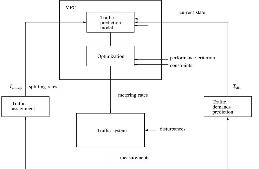
Fig. 4. Schematic representation of the anticipative MPC-based control strategy for ramp metering.
