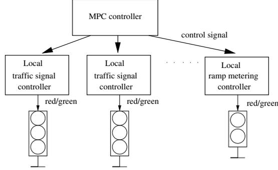
Figure 7: MPC-based control implemented with local controllers
