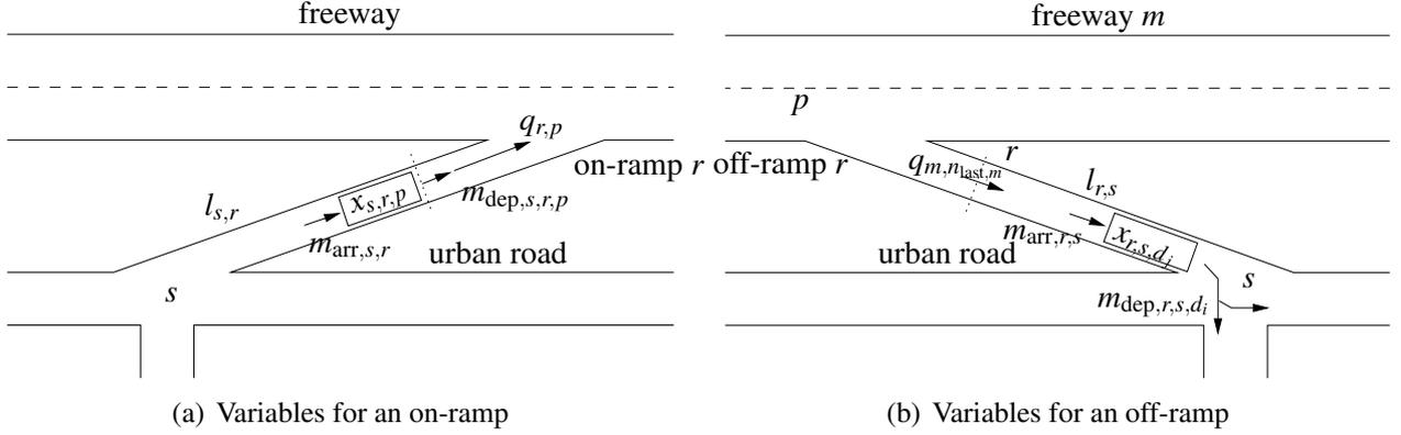
Figure 4: Overview of variables on on-ramps and off-ramps
