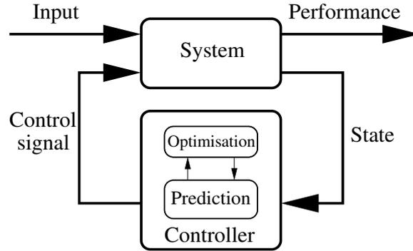
Figure 6: Working principle of MPC
