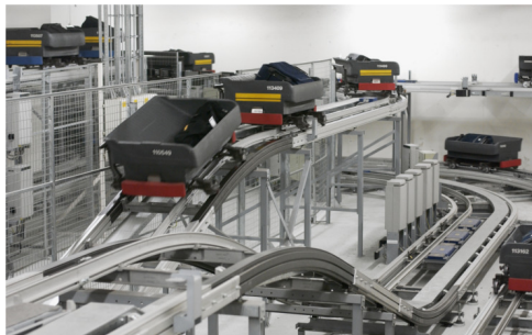
Fig. 1 DCVs running on a network of tracks (Photo courtesy of Vanderlande Industries)
