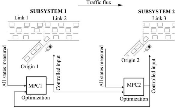
Fig. 2. Distributed MPC for the case of study
