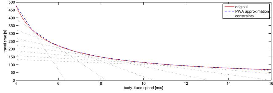
**Fig. 5** Travel times at different speeds. The convex function can be approximated using constraints.
