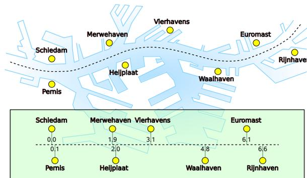
**Fig. 1** The micro-ferry scheduling problem for the Rotterdam harbor: find an energy-efficient schedule for transporting people between stations along the river. The distances (in kilometers) of the stations along the river are indicated in the lower plot.
