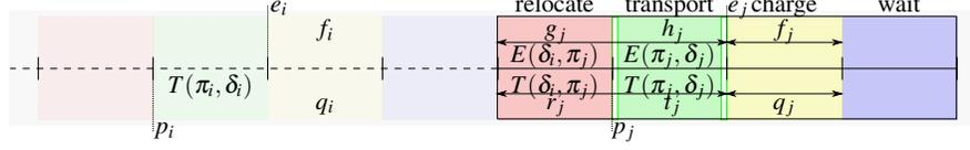
**Fig. 7** The four phases of a request consist of relocating, transporting, charging, and waiting. The associated energy (top) and time (bottom) variables show the relations between energy levels  $e$  and pick-up times  $p$  for successive requests.
