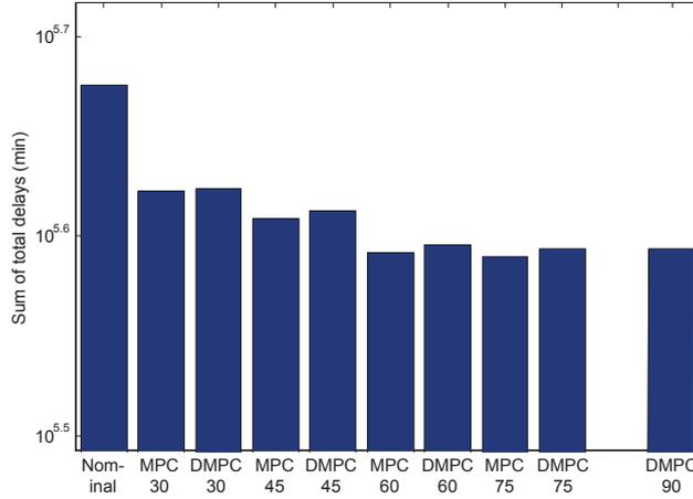
Figure 5: Sum of delays of all scenarios for DMPC 2.2 and the global MPC approach for prediction horizons of length 30, 45, 60, 75, and 90 minutes.
