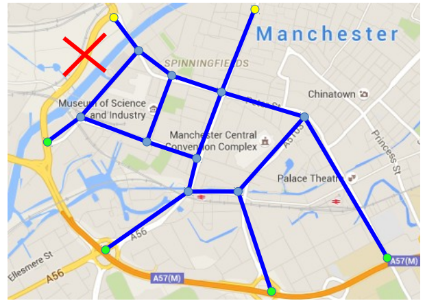
Figure 4: The considered scenario B. It represents a section of the Manchester urban area. Modelled roads are shown in blue. Part of the ring road (crossed out) is blocked. Incoming traffic flows enter the network from entry points (green) and have to reach exit points (yellow).
