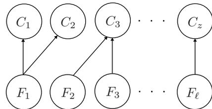
Figure 3: Bayesian network representation of the knowledge-based fault diagnosis problem. The variables  $F_1$  till  $F_\ell$  represent the different system faults and the variables  $C_1$  till  $C_z$  are the diagnostic features.
