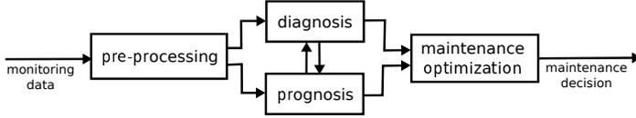
Figure 2: Fault diagnosis within the condition-based maintenance process.
