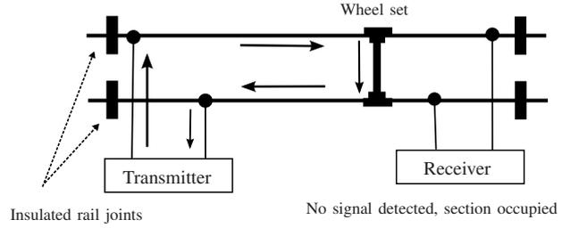
Fig. 2: Flow of current in a railway track circuit.
