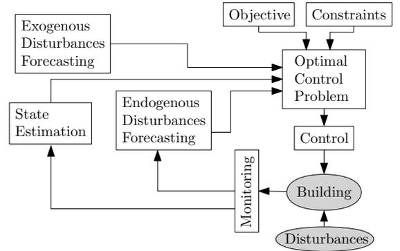
Fig. 2. Scheme of the MPC framework [10].
