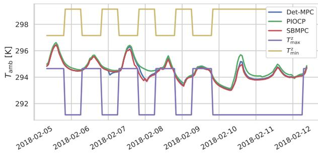
Fig. 5. Simulation profile of the room temperature evolution of one winter week with the three different methods considered in Section V.  $T_{\max}^z$  and  $T_{\min}^z$  stand for the maximum and minimum comfort temperature, respectively.
