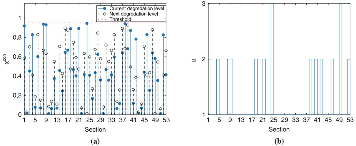
Figure 5: Simulation results for the whole railway network at representative time step ( $k = 6$ ). (a) Degradation levels of the whole railway network at time step 6 (current time step) and time step 7 (next time step). (b) Interventions suggested by the high-level MPC controller at time step 6 for the whole railway network.
