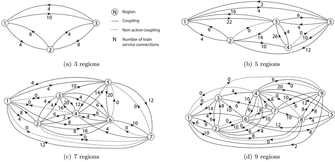
Figure 5. Railway network decomposition (GEO decomposition) in the cases of 3, 5, 7, and 9 regions
