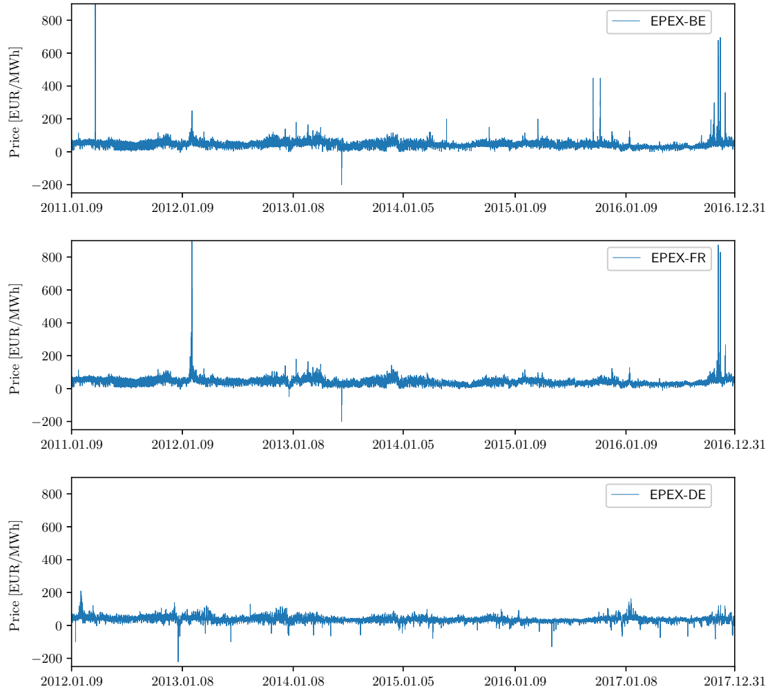
Figure 3: Electricity prices time series for three of the five datasets, i.e. EPEX-BE, EPEX-FR, and EPEX-DE, considered in the open-access benchmark dataset (Note that each dataset also includes two exogenous time series that are not plotted here). The EPEX-BE and EPEX-FR time series are similar because the EPEX-FR and EPEX-BE are highly coupled markets [43]. To keep the plots readable, the upper limit of the y-axis is below the maximum price; this only affects one spike in EPEX-FR and another one in EPEX-BE.
