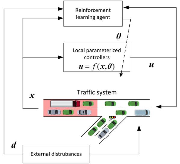
Fig. 1. The diagram of the proposed RL-based adaptive parameterized controller
