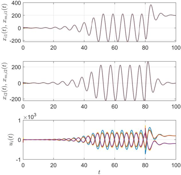
Fig. 9. Example 3: States and control inputs of the agents under the proposed MRASCon law (22) with switching reference models (unstable for  $t \leq 50$ ; marginally stable for  $50 < t \leq 80$ ; stable for  $t > 80$ ).
