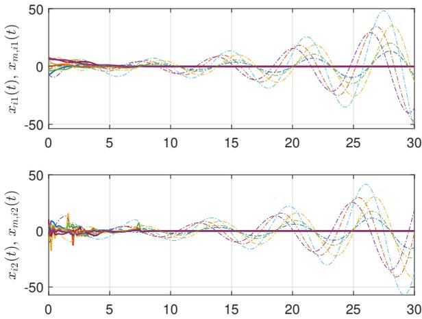
Fig. 6. Example 2: States of the agents under MRACCon\* law (obtained by removing  $F_i(t)e_i$  in MRASCon (22)). The agents (solid lines) reach a trivial consensus at zero, but fail to track the corresponding local reference models (dashed lines): that is, a trivial consensus is reached without tracking.
