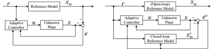
Fig. 1. Block diagrams of MRAC (left) and CMRAC (right). CMRAC modifies the original reference model: the modified closed-loop reference model plays a role of an observer of the original reference model.
