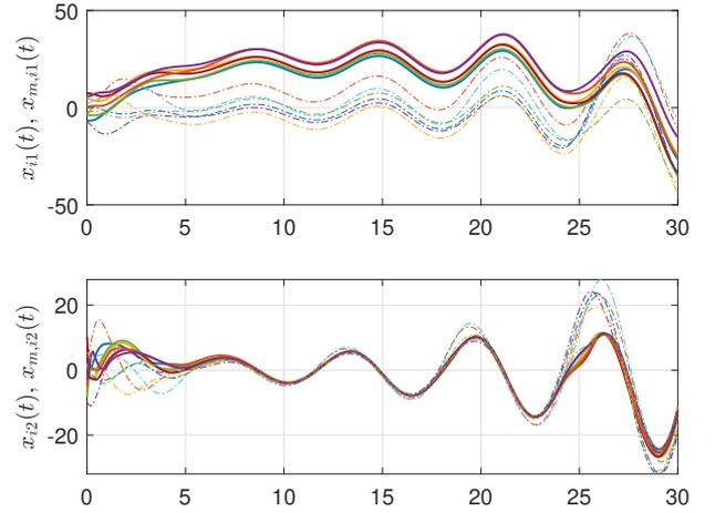
Fig. 7. Example 2: States of the agents under CMRACon law (31) with  $\rho = -100$ . The agents (solid lines) fail to accomplish the consensus and tracking tasks.
