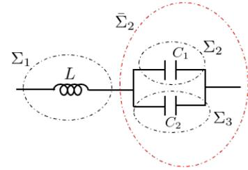
Fig. 2. The interconnection  $\bigwedge_{i=1}^3 \Sigma_i$  is not a regular feedback interconnection; however, if merging  $\bar{\Sigma}_2 = \Sigma_2 \wedge \Sigma_3$  into a single component,  $\Sigma_1 \wedge \bar{\Sigma}_2$  becomes a regular feedback interconnection of two components.
