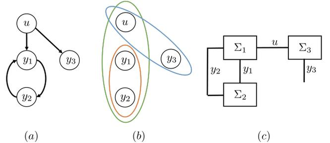
Fig. 3. A directed graph of an SVAR model is shown in (a). The model also defines an interconnected system in the behavioral setting with a signal graph (b) and a system graph (c).
