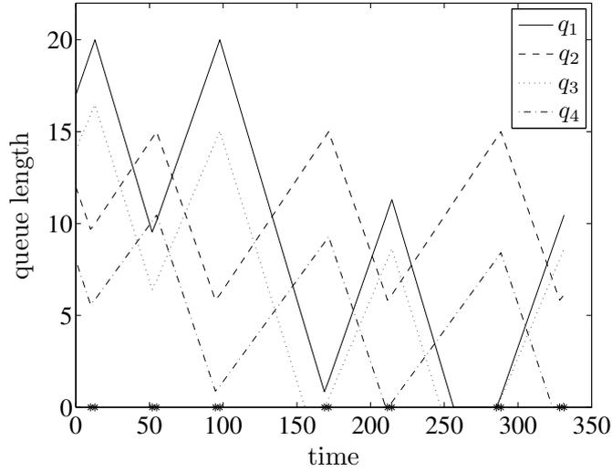
Figure A.2: The queue lengths in the various lanes as a function of time for the traffic signal switching sequence that corresponds to the switching interval vector  $x_{\delta, \text{elcp}}^*$  of the example of Section 5.2. The \* signs on the time axis correspond to the switching time instants.
