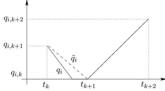
Figure A.1: The functions  $q_i$  (full line) and  $\tilde{q}_i$  (dashed line) for a queue with a decrease phase and a subsequent positive growth phase and without saturation at an upper level. Note that in the growth phase the functions  $q_i$  and  $\tilde{q}_i$  coincide.
