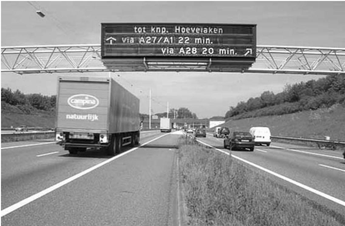
*Figure 2.5: A route guidance system showing travel times for alternative routes to a common node.*
