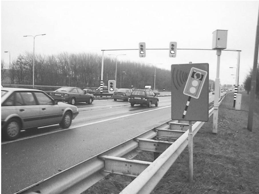
*Figure 2.1: Ramp metering at the A13 at Delft in The Netherlands. One car may pass per green phase. To prevent red-light running the control is enforced.*
