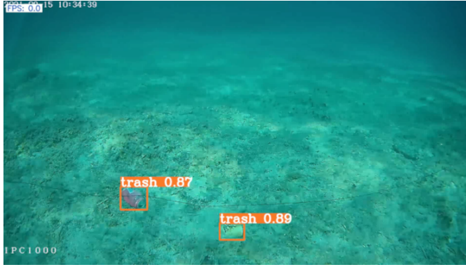
Figure 4.8: Example result of the YOLO object detection algorithm.
