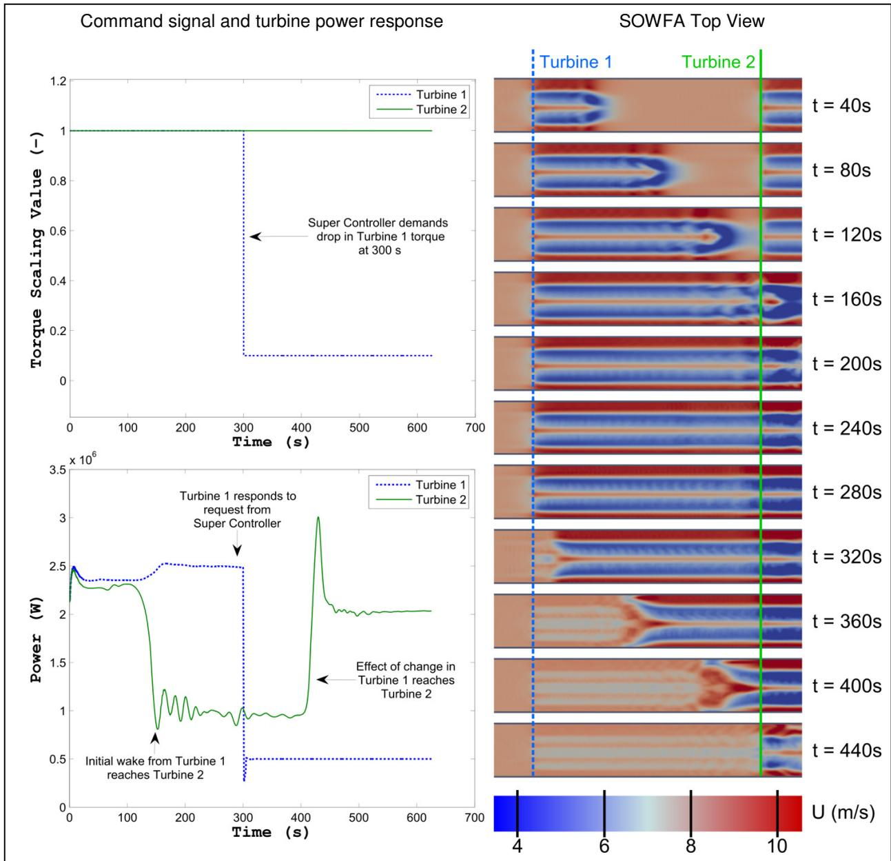
Figure 5. Results of a step response simulation with SOWFA for a two-turbine setup.
