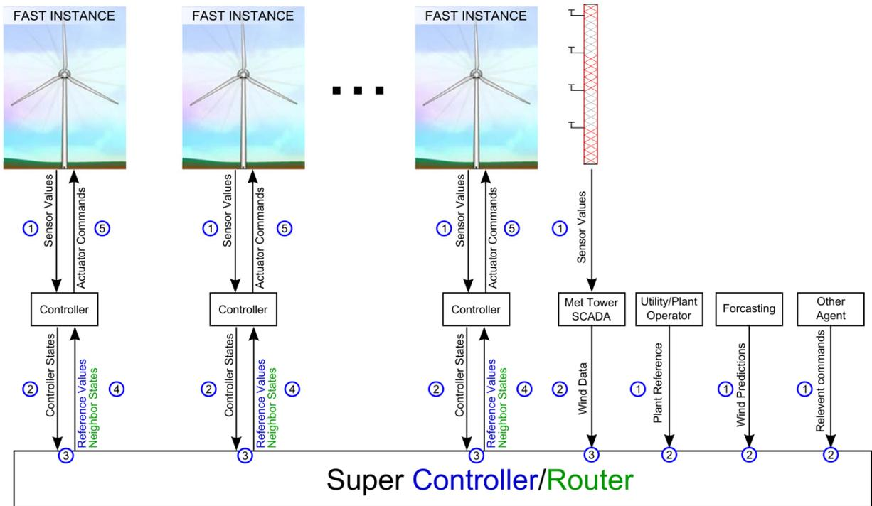
Figure 2. Control architecture in SOWFA.
