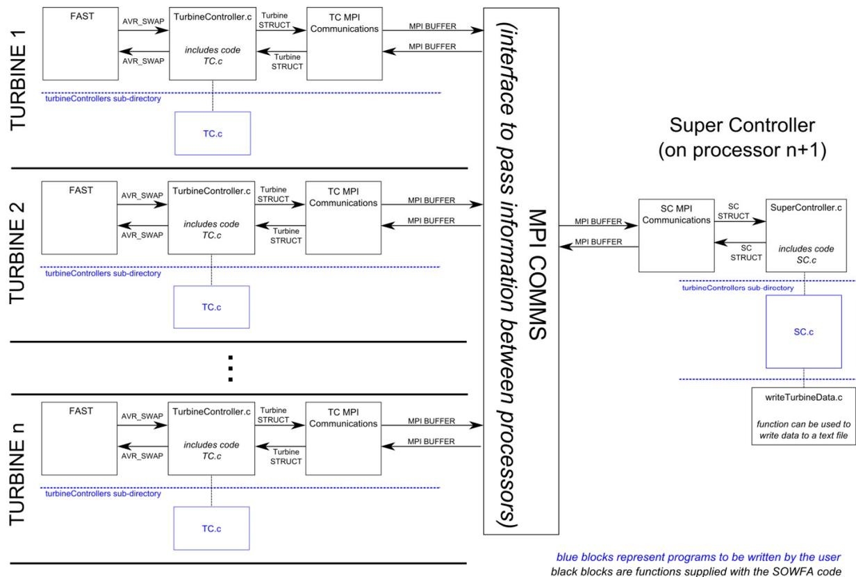
Figure 3. Communication in the SOWFA super-controller architecture.
