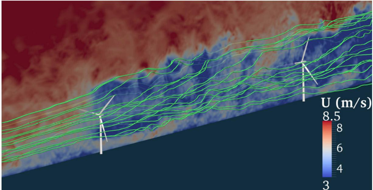
**Figure 1. SOWFA simulation of two turbines subjected to an atmospheric boundary layer. The streamlines show the instantaneous velocity contours [24].**
