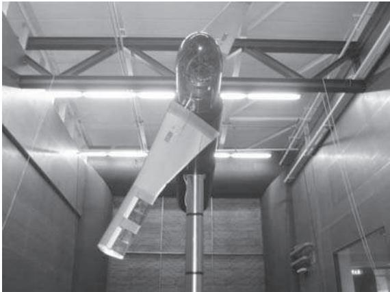
Figure 2: “Smart” rotor scale model in the Open Jet facility.
