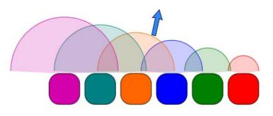
Such a system is more fit for the communication between air-planes and satellites. However, a socalled beam-former is needed to control the delays at each antenna. It essentially steers the antenna, but electronically instead of mechanically. Usually,ma beam-former is an electronic device.
