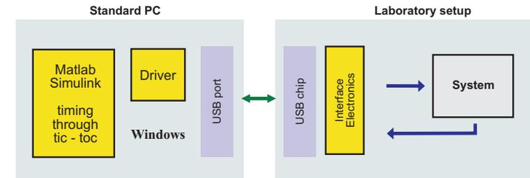
Possibly more sampling period jitter in the beginning of experiment – in case of suspicion, discard a few initial samples.
