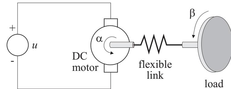
Abstraction of many real-world systems, such as robot arms, motors with gears, etc.
