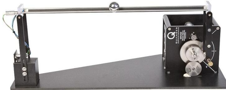
Figure 1: Photo of the ball and beam setup.
