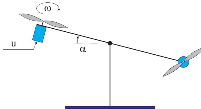
Figure 1: Schematic drawing of the helicopter setup.
