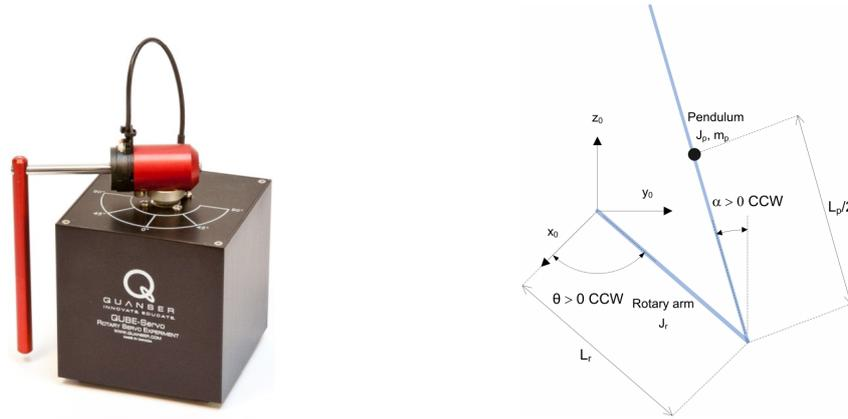
Figure 1: Qube-Servo setup and its schematic representation.
