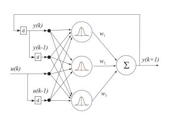
Another possibility would be a multilayer neural net. In the above scheme, the 'd' block denotes the delay operator. The output of the network is the predicted output of the dynamic system y(k + 1). The inputs of the network are y(k), y(k - 1) (obtained by delaying the output) and u(k), u(k - 1), where u(k) is the given input to the dynamic system and u(k - 1) is the one step delayed value of this input.
