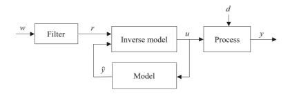
The reference-shaping filter generates the desired dynamics in order to avoid peaks in the control action for step-wise references.
